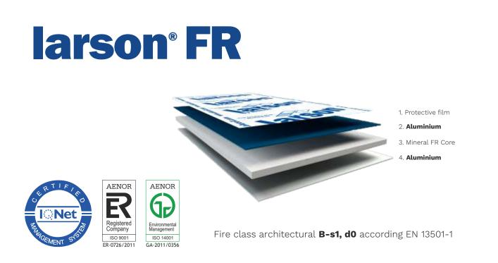
**larson® FR** aluminium composite panel, is a high-tech product for architectural façade cladding. It is formed with two aluminium sheets, 5005 alloy, bonded by a mineral fire retardant (FR) core. **Alucoil®** has developed a core that delays panel combustion which allows this material to achieve **B-s1**, **d0** classification, according to the EN 13501-1 standard.
